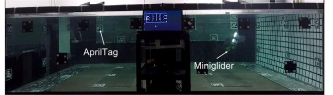
Fig. 6. Miniglider robot operating in a large indoor tank during experiment. Onboard sensors are used to estimate body-fixed velocities, while AprilTags and onboard camera are used to localize the robot.
