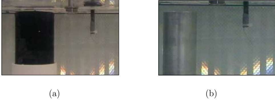
Figure 6.13: IPMC sensor was attached behind of the: (a) 6 cm diameter cylindrical obstacle; (b) 4 cm diameter cylindrical obstacle.
